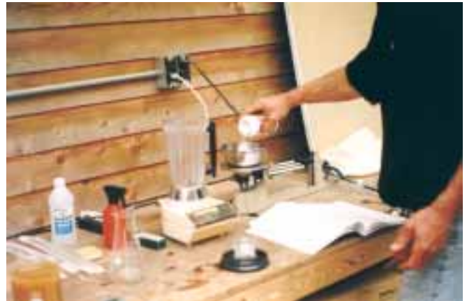
Measuring lye for the test batch. The red spray bottle contains an acidic vinegar solution to neutralize any spilled lye.
