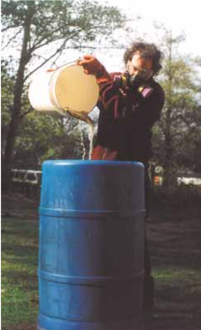
Scott Durkee going for a big batch—adding the sodium methoxide to the used vegetable oil that will soon be biodiesel fuel for his Mercedes 240 D.
